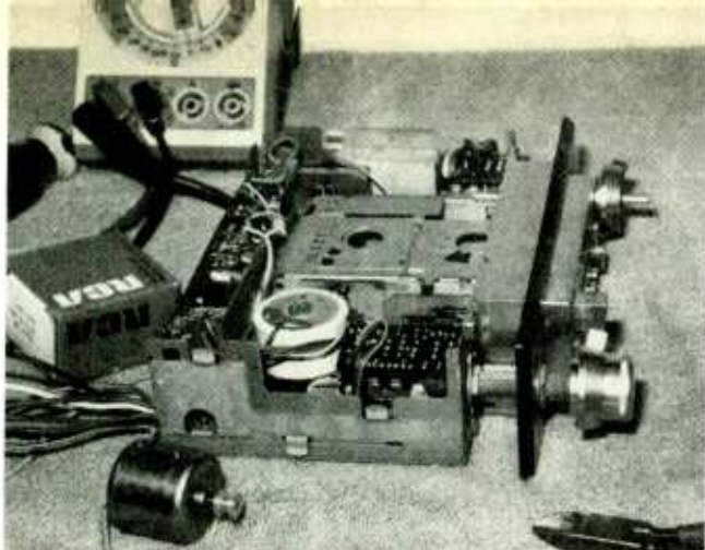
Fig. 2—Check the cassette switch and isolation resistor when no voltage is found at the motor terminals. Replace the motor if tape movement is erratic or intermittent.
